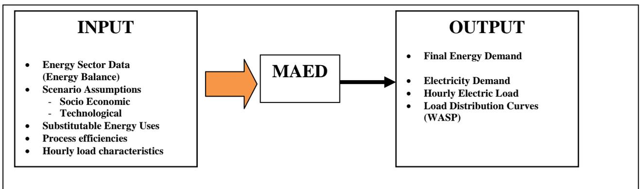
Figure 1 : Main Inputs and Outputs of MAED
